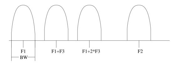
In the FSCAN the first measurement occurs exactly on the start frequency. The next measurements occur at the frequencies Fn (F3 = step frequency) :
